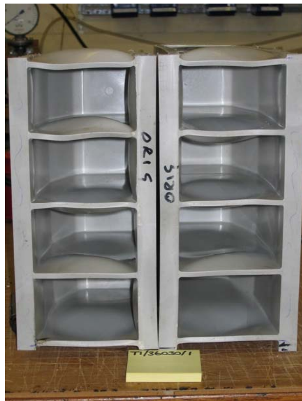
Photograph 3. Distortion of internal rib supports after compressive strength.
